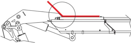
Second boom with negative angle in order to simplify operations in difficult access conditions
